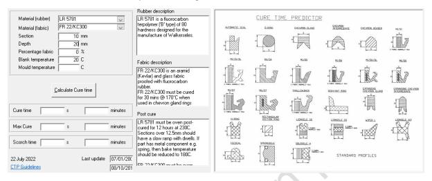
4.8 If applicable enter **Fabric Percentage** based on the finished part drawing / moulded profile dimensions. See example profiles for **Fabric Percentage** guidance.
